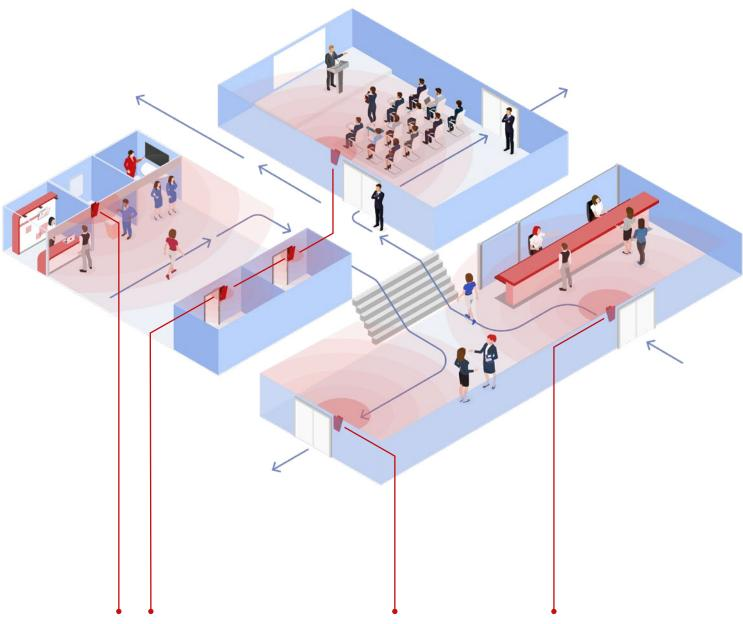
The Track Boxes are positioned at key locations such as lecture halls, staff rooms, cafeterias, or highly frequented areas. Hotspots can be identified and a simple student count and alert system can be implemented. Transponder flows can be recorded and possible contact persons can be traced afterwards.
